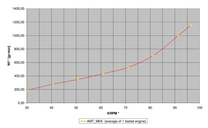
SFC VS. RPM, corrected to STP MK - 6
